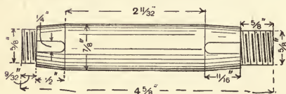
Fig. 66.—Main Shaft, Pulley Side.
