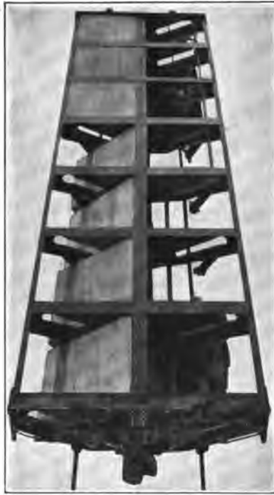
FIG. 61.—Underframe of drop-bottom convertible stock car.
