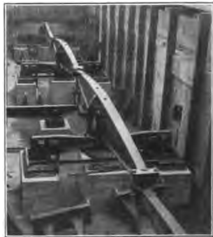
FIG. 67.—Lever arrangement, track scale—Baltimore & Ohio.
