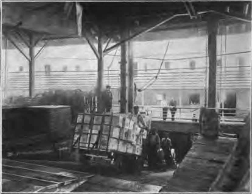
FIG. 158.—Electric freight truck unloading vessel.
