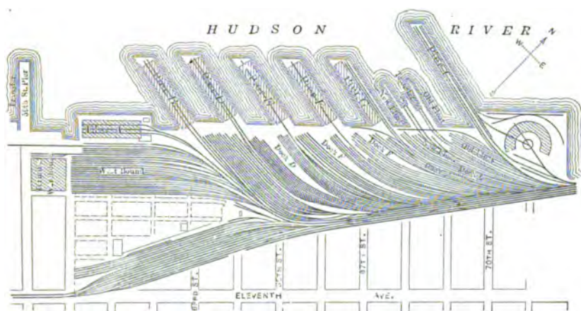
FIG. 78.—Plan of yards and piers, East 69th Street, New York City—New York Central.
