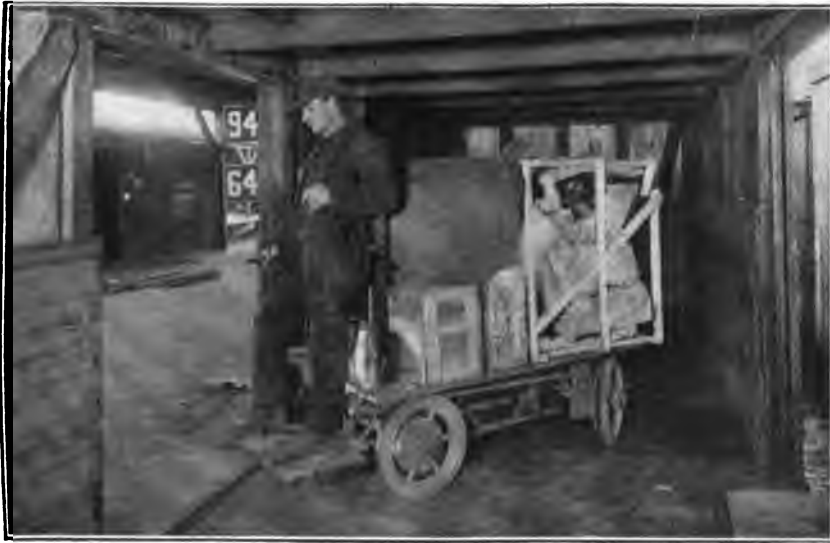
FIG. 156.—Electric freight truck, loaded, inside a box car.
