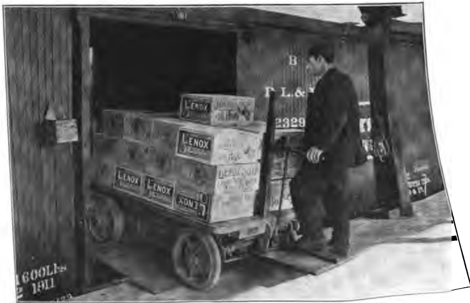
FIG. 157.—Electric freight truck entering a box car.
