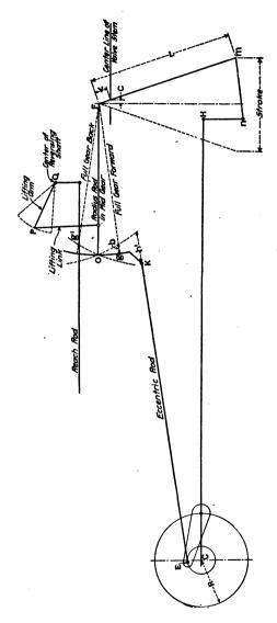
Fig. 29.—Reference Diagram, Walschaert Valve Gear.
