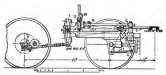
Fig. 10.—Mason's Improved Design of Walschaert's Valve Gear.
