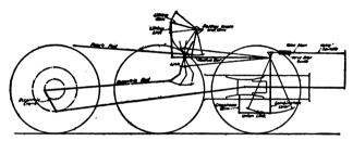
Fig. 13.—Diagram of Valve Gear, Low-Pressure Gear, or Forward Section of Mallet Compound Locomotive.
