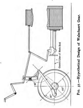
which the eccentric is placed must always be 90 degrees from a line through the hub centre and link-foot pin when the link is in an exactly vertical position—a position in which the reverse lever can be moved
