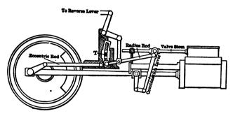
Fig. 6.—Building up the Walschaert Valve Gear.
