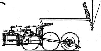
Fig. 7.—Walschaert Valve Gear Complete. Sectional elevation of valve and cylinder.
