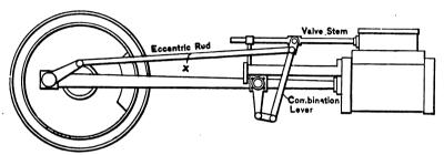
Fig. 5.—Simple Form of Steam Engine with the Walschaert method of Providing Lead.
