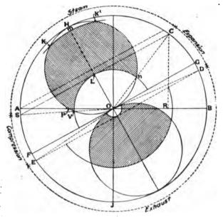
Fig. 33.—Combination of the Reauleaux and Zeuner Diagrams.
